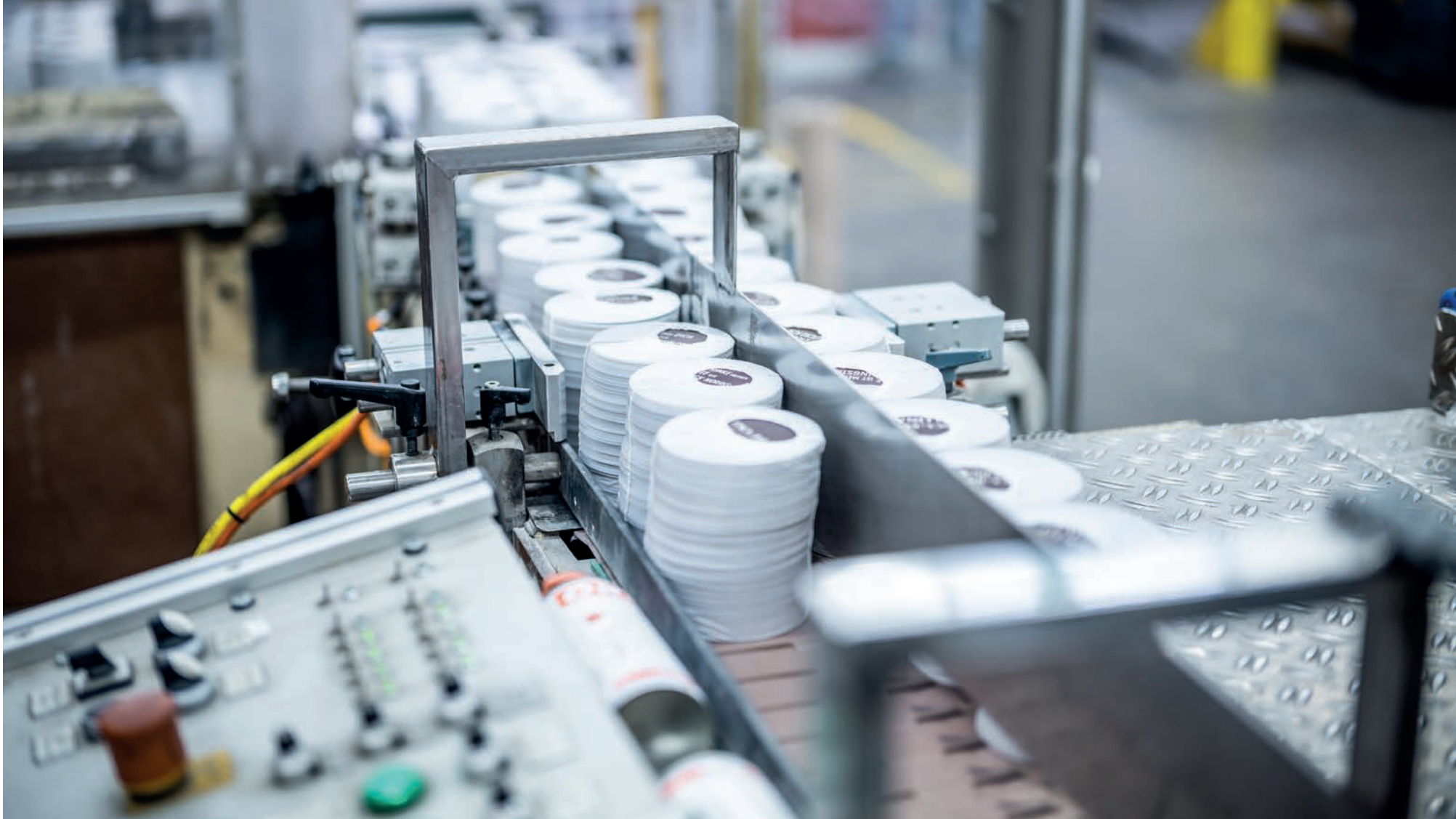
View of the packaging of printed beverage coasters into rolls.
